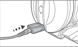
3. Connect the external adaptor to the power source. The indicator light on the external adaptor will turn red when the vacuum is charging and green when it is fully charged. Charge it for 5-6 hours for best performance.
