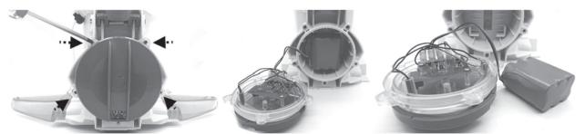
2. To detach the battery connection wire, press on the clip of the connector to pull it out. NOTE: Wrap the connector immediately with insulating tape in order to avoid any short circuit caused by the contact of both wire terminals.
