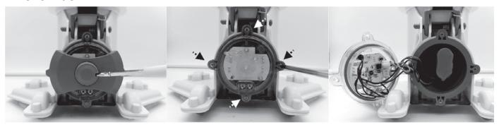
2. Remove the battery from the unit and locate the battery cable connector. Press on the clip of the connector to pull it out. NOTE: Wrap the connector immediately with insulating tape in order to avoid any short circuit caused by the contact of both wire terminals.
