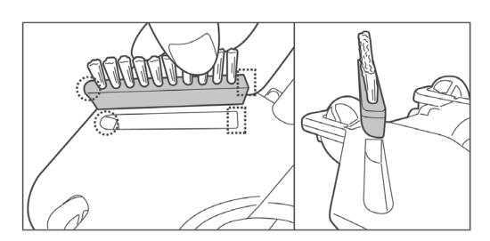
To detach the brush, insert the tip of a small screwdriver into the corner notch and pry up the brush.
