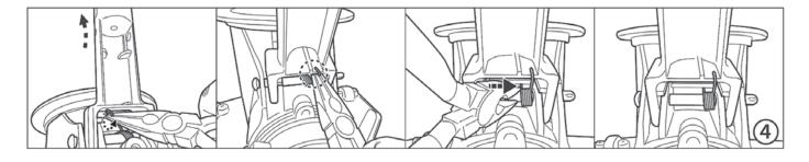
4. Use a pair of pliers to pull the hook from the bottom of the connector, then fix it onto the connector as shown. Move the entire spring to the right.
