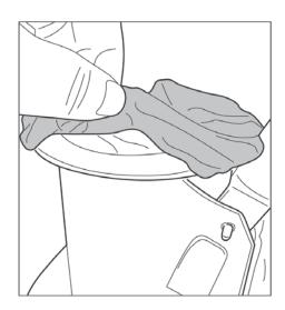
Spread the filter bag over the top opening of the main body of the pool vacuum. Make sure the cord of the bag is placed under the flange of the top opening.
