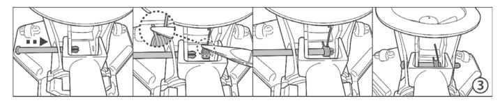
3. Insert the pin from one end and place the spring as shown with the help of a pair of pliers. Ensure the hook is on top and the other end is installed underneath the bench as shown. Align and insert the pin all the way through the spring hole and opposite hole.
