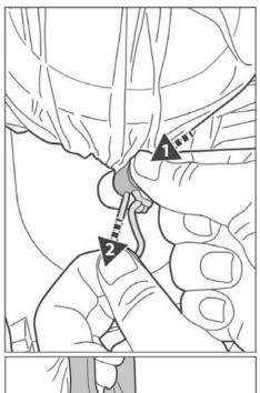
While holding the cord, press on the cord fastener and push it under the flange.
