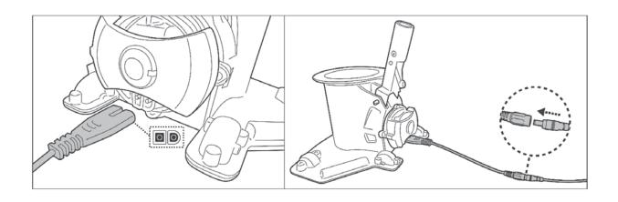
3. Connect the external adaptor to the power source. The indicator light on the external adaptor will turn red when the vacuum is charging and green when it is fully charged. Charge it for 5-6 hours for best performance.
