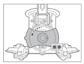
2. Align and attach the charging cable to the charging port. **WARNING!** Be sure not to invert the charging cable and ensure both the charging cable and charging port are clean and dry before charging them. TIPS: Use cotton bud to dry the charging port and pins. Connect the external adaptor's cable plug to the charging cable's port.
