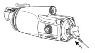
4. Connect the external adaptor to the power source. Once the pool vacuum begins charging, the indicator light on the external adaptor will turn red. Normally, it takes about 4-6 hours to reach a full charge. The indicator light will turn green when the pool vacuum is almost fully charged.
