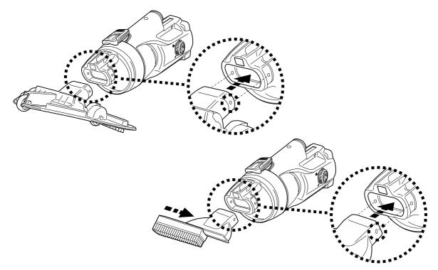
NOTE: To replace the brushes on the suction head, lift the end and pull it out to make space for a new one.
