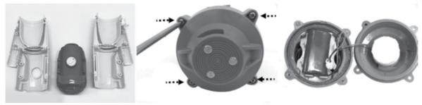
4) Use Philips screwdriver to unscrew screw on the corner of the supporting plate as pointed at. Use clamp to catch the plate and pull it out to expose the wire connectors on the PCB.
