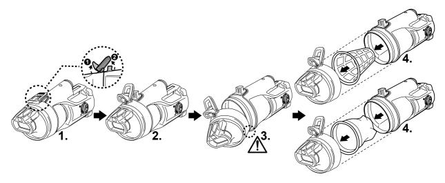
**CAUTION!** Replace the damaged filter bag/filter cage immediately before the next operation.
