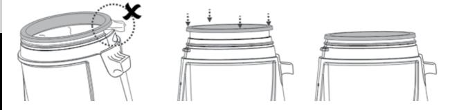
To re-install the canister, first align the notch of the canister with the hook on main body and then press the canister onto main body. Align the latch bolt to the catch and press down the lever completely to secure the locking.
