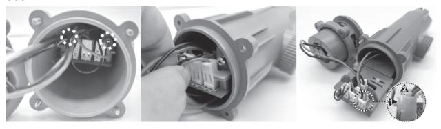
3. Use the screwdriver to unfasten the 4 screws on the PCBA. Remove the PCBA to expose all wire connectors. Release the middle wire connector in the first row. Cut the tape and remove the battery. Wrap the connector of the battery immediately with insulating tape in order to avoid short circuit caused by contact of both wire terminals.
