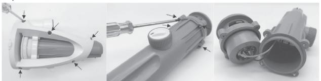
Use the screwdriver to unfasten the screw on the corner of the support plate. Pull out the plate to expose all wire connectors. Detach the wire connector at the corner as shown by pressing on its clip and pulling it out.
