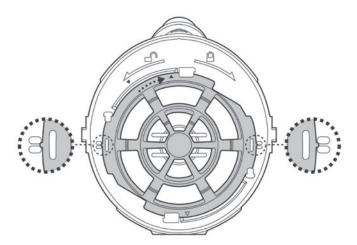
7. Align and re-assemble the hood to the pool vacuum and make sure the lever is secured by pushing it down all the way to the hood.
