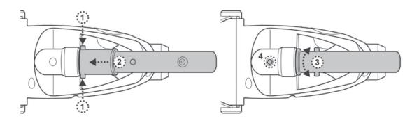
Slide the telescopic pole onto the pole connector. Press on the side pins of the connector and slide the telescopic pole further down until the pins of the connector are secured inside the holes of the pole.
