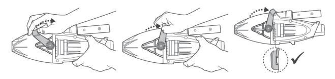
3. Detach the hood and carefully unhook the socks from the filter cage. Remove the sock and turn the filter cage anticlockwise until triangular indents are aligned. Take the filter cage out of the cleaner.
