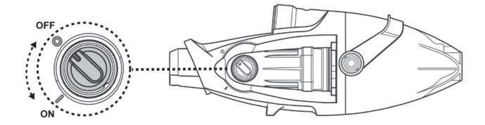
2. Pry open the protective cap. Align and attach the charging plug to the charging port.
