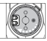
DO NOT cover the side slot (middle gap) of the electric vacuum during operation, the impeller / motor may be damaged otherwise.
