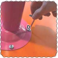
STEP 2: Use provided allen key to screw in your 4 retaining bolts. Tighten until snug. Do not overtighten.
