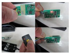
Step 5. Carefully put the circuit board back into the external black plastic box and ready to use the remote control function.
