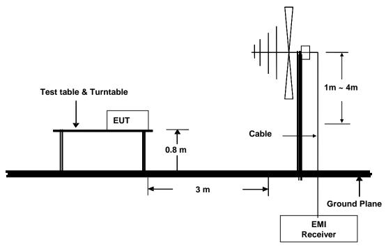
The EUT was placed on a wooden turntable which could rotate from 0° to 360°, 0.8m high above the ground, the distance between the EUT and the antenna is 3m.
