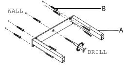
**3.** Optional: Install two phillips wood screws **(B)** through the interior metal tubes **(A)** into the shelf ceiling. This locks the shelf in place on the bracket.
