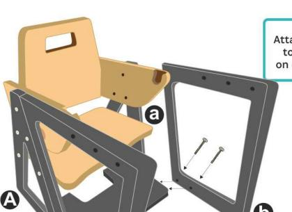
Attach the bottom side frame **B** & **b** to the foot rest using two screws on each side as shown un the figure
