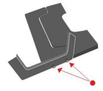
Don't tighten the screw fully. Only after the complete assembly, the screw has to be tightened finally
