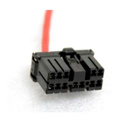
The internal multicontroller board provides a single differential CANbus port accessible through screw terminals on one end. These connections are wired to the Tesla Model S diagnostics port mating connector through a cable that exits the enclosure through a weatherproof gland nut on one end.
