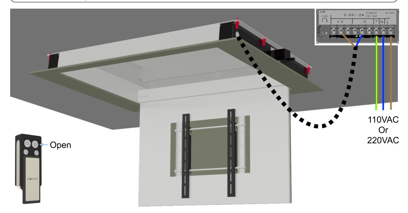
Connect the power supply to a power source 110v or 220v.
