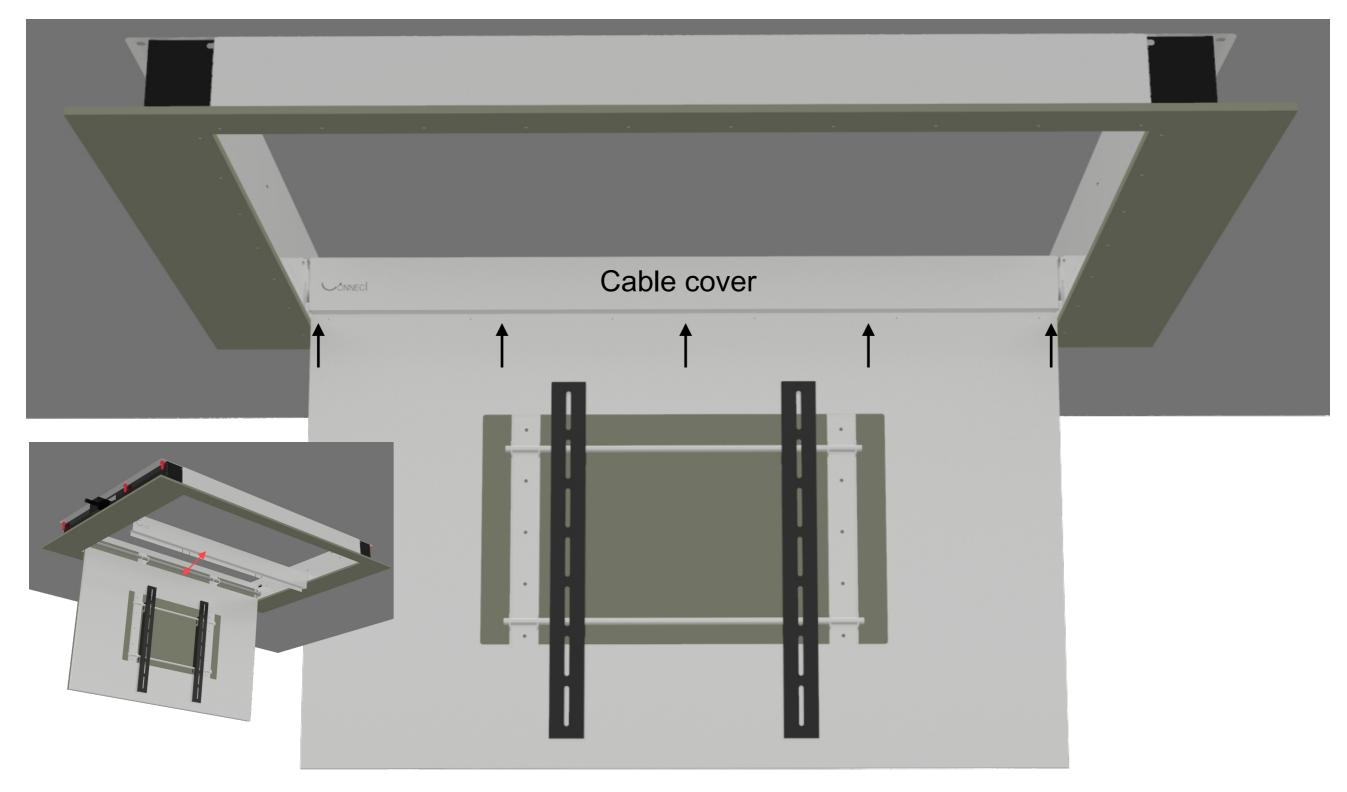
Loosen the screws of the cable cover
