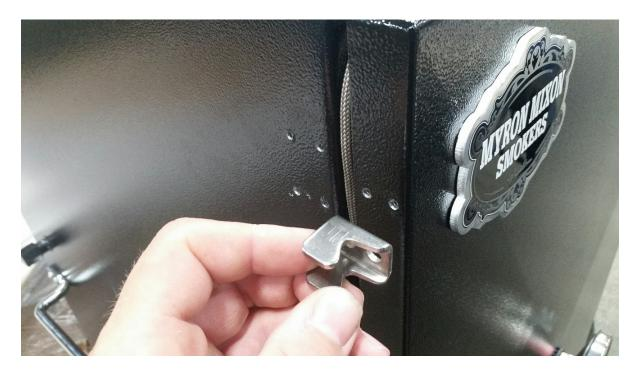
5. Install new catch and tighten screws.
