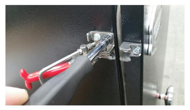
7. Test operation and adjustment of clamp. Adjust clamp if necessary.
