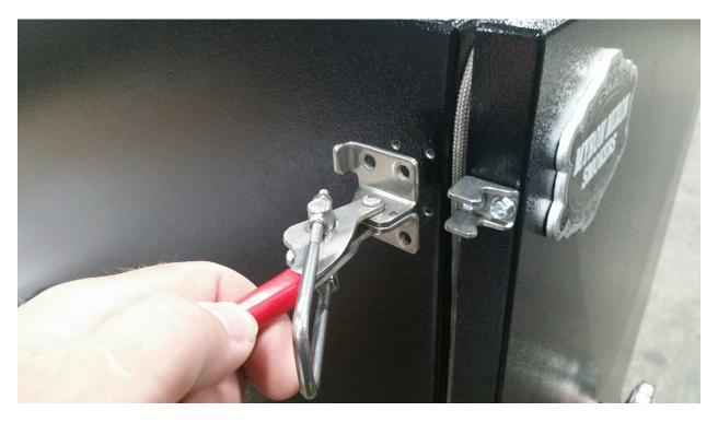
3. If catch needs to be replaced, remove the 2 screws securing it to the door. If the catch does not need replacing, skip to step 6.
