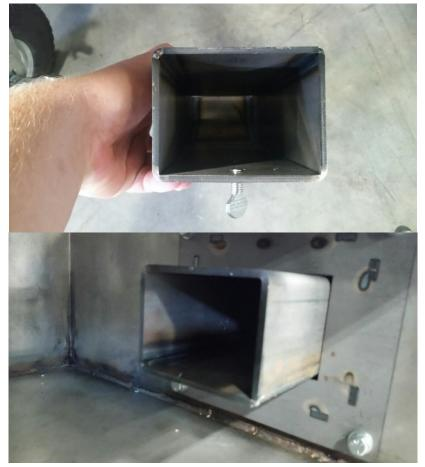
4. Reinstall transfer chute and tighten thumb screw.
