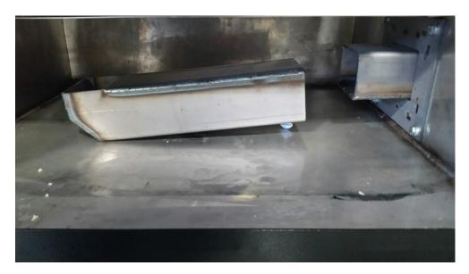
3. Empty ash out of the transfer chute and clean any ash out of the tube sticking into the cook chamber from the fire box. Store and dispose of ash properly.
