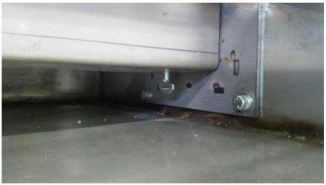
3. Loosen the thumb screw and remove the transfer chute.
