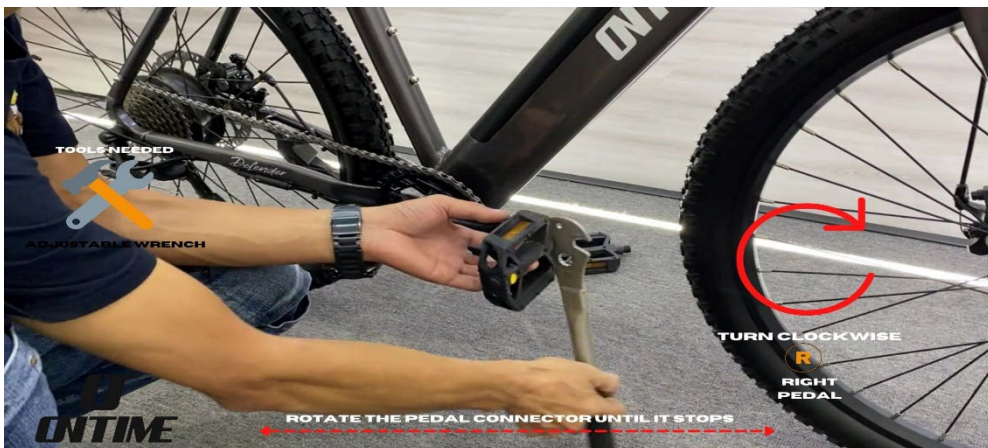
tightening bike pedals [Right Pedal – Clockwise / Left Pedal – Counter-Clockwise]
