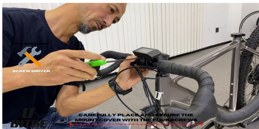
Secure the handlebar mount cover with the four screws
