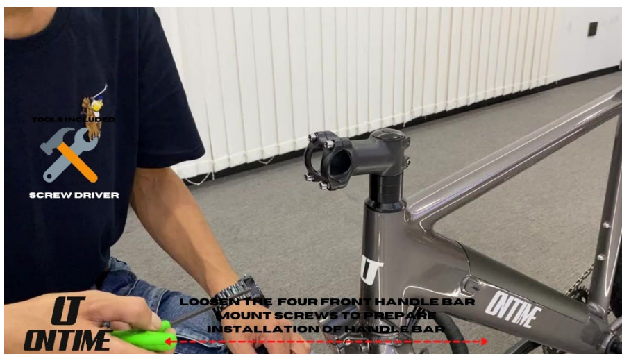
Loosen the four handle bar mount screws
