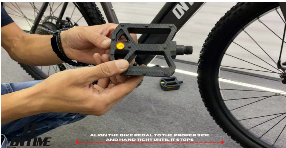
Align bike pedals with bike pedal threads
