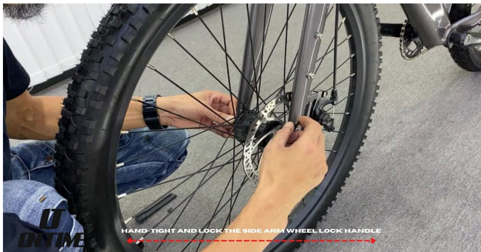
Secure both side front wheel bolts
