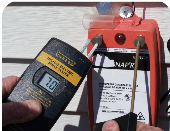
Reading voltage of the power controller while disconnected from the system.
