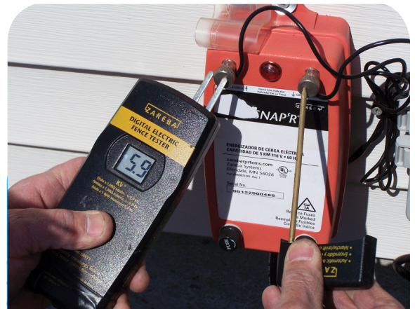
Reading voltage with the entire Shock-Tape system connected.
