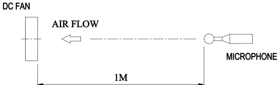
NOISE IS MEASURED AT RATED VOLTAGE IN FREE AIR IN ACOUSTICAL CHAMBER WITH LARSON DAVIS TYPE 824S SOUND LEVEL METER.
