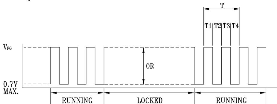
$$T = T_1 + T_2 + T_3 + T_4 = 60/N \text{ (Sec)}$$
