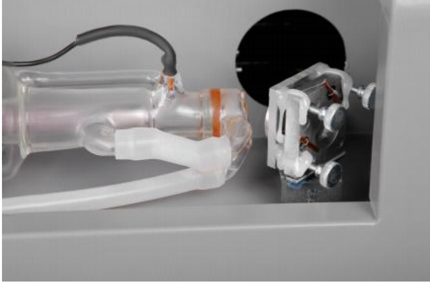
Fig. 5 - 2 - Adjustment set screws Behind the First Mirror
