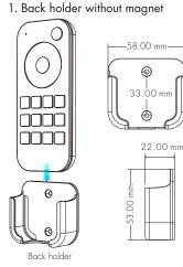
**Back holder** Two options are offered for selection, please fix the back holder on the wall with two screws, or adhere the back holder to the wall with paster.
