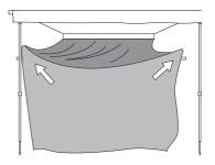
STEP 5 Zip the two sections together. It may be necessary to release the tension on the awning rafter arms to get the zip started.
