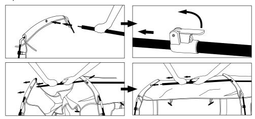
Insert the trigger lock spreader pole into one of the centre eyelets. Release the trigger to extend the pole and insert into one of the end eyelets. Tension the bar to stretch the swag into shape then lock into position. Repeat this process for the other spreader pole. The guy ropes and pegs can be used if required.
