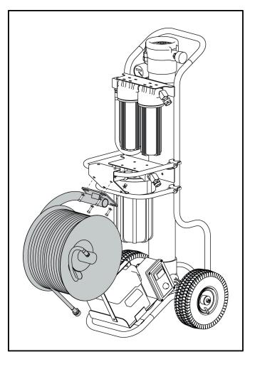
2. Attach hose reel assembly to hose reel bracket with (4) bolts, (8) flat washers and (4) Nylock nuts.
