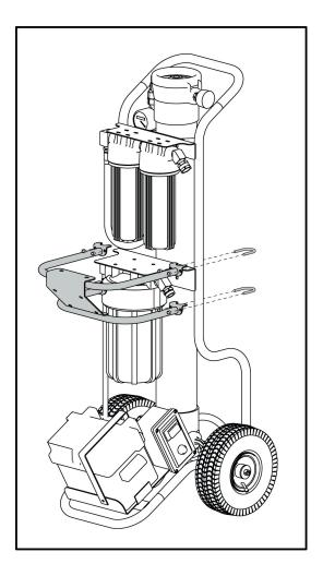
1. Attach on hose reel mounting bracket to cart frame with the (4) U-bolt assemblies.
