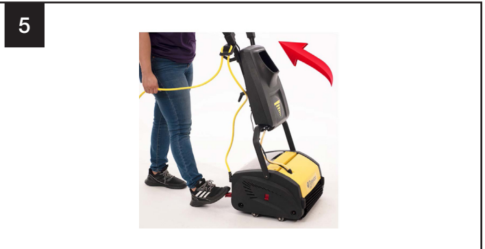
Start the machine by pressing the handle release pedal and pulling the handle back.
