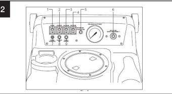
Turn the heater switch (#2) to the "ON" position. Note: The orange indicator light (#8) is on any time the heater is operating.
