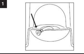
If you are not pre-spraying the chemical on the carpet, fill up the fresh water solution tank with tap water that is no hotter than 135° F (57° C) and approved carpet cleaning chemical, following the mixing instructions for the chemical being used, into the solution tank. If using the EZ Fill hose option, remove the hose from the solution tank and connect the hose to a water faucet.
