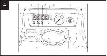
Turn the pump switch (#1) to the "ON" position.
