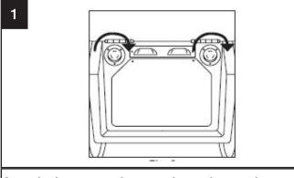
Attach the extension cords to the sockets on the back of unit and twist clockwise to lock in place.
