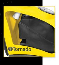
PATENTED BLADDER DESIGN — The Marathon bladder system maintains a constant level of brush pressure for optimal extracting performance at all fluid levels.
