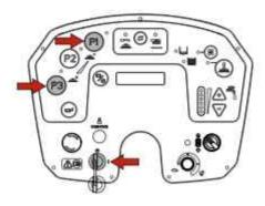
Press the programming button three times, the message "GEL battery" will appear on the display.
