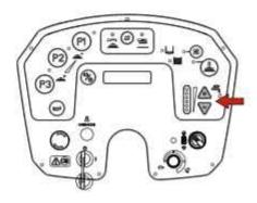
Store the parameter by pressing and holding the programming button until the display shows the battery voltage value.
