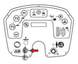
Press the brush attach/release button; the machine will respond by operating the release mechanism.
