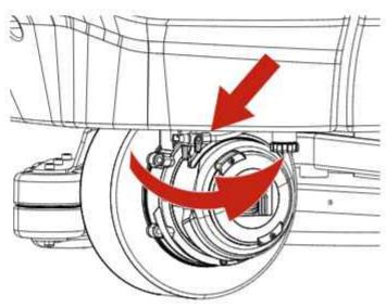
Unscrew the filter cap, remove the filter, then wash under running water or using the same detergent dispensed by the machine.
