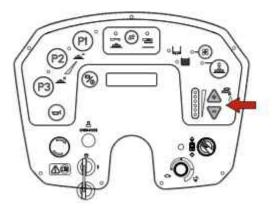
To store the changes and exit, press and hold the programming button until the display shows the battery voltage.
