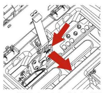
Rotate the stop, and release the knob so that it locates in the retaining hole:
