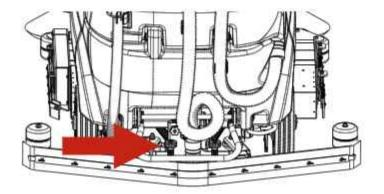
Connect the vacuum hose to the squeegee, bending it to the position as illustrated.
