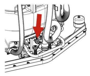
Similarly, the height of the squeegee can be adjusted by raising or lowering the two wheels positioned in front of / behind the squeegee, turning the relative knobs.
