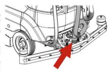
Tighten the two knobs.
