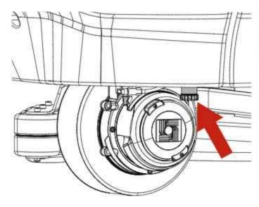
Replace the filter in its housing, making sure it is correctly positioned and screw the lid back on.
