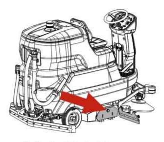
Position the roller brushes in the two compartments, making certain that the guide pin on the opposite side is correctly located.
