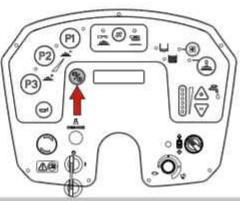
Press the programming button until the parameter "Chemical flow rate" appears.
