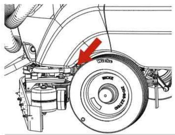
Unscrew the filter cap, remove the filter, then wash under running water or using the same detergent dispensed by the machine.
