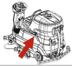
or use the hose with ACQUA-STOP fill system (model with ACQUA-STOP). Once the quick coupling hose is connected to the machine, this device allows the tank to be filled without the presence of the operator. Dispensing will be stopped automatically when the tank is filled.
