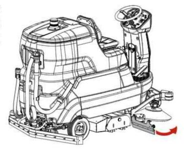
Remove the cover from the brush compartment by unscrewing the knob.
