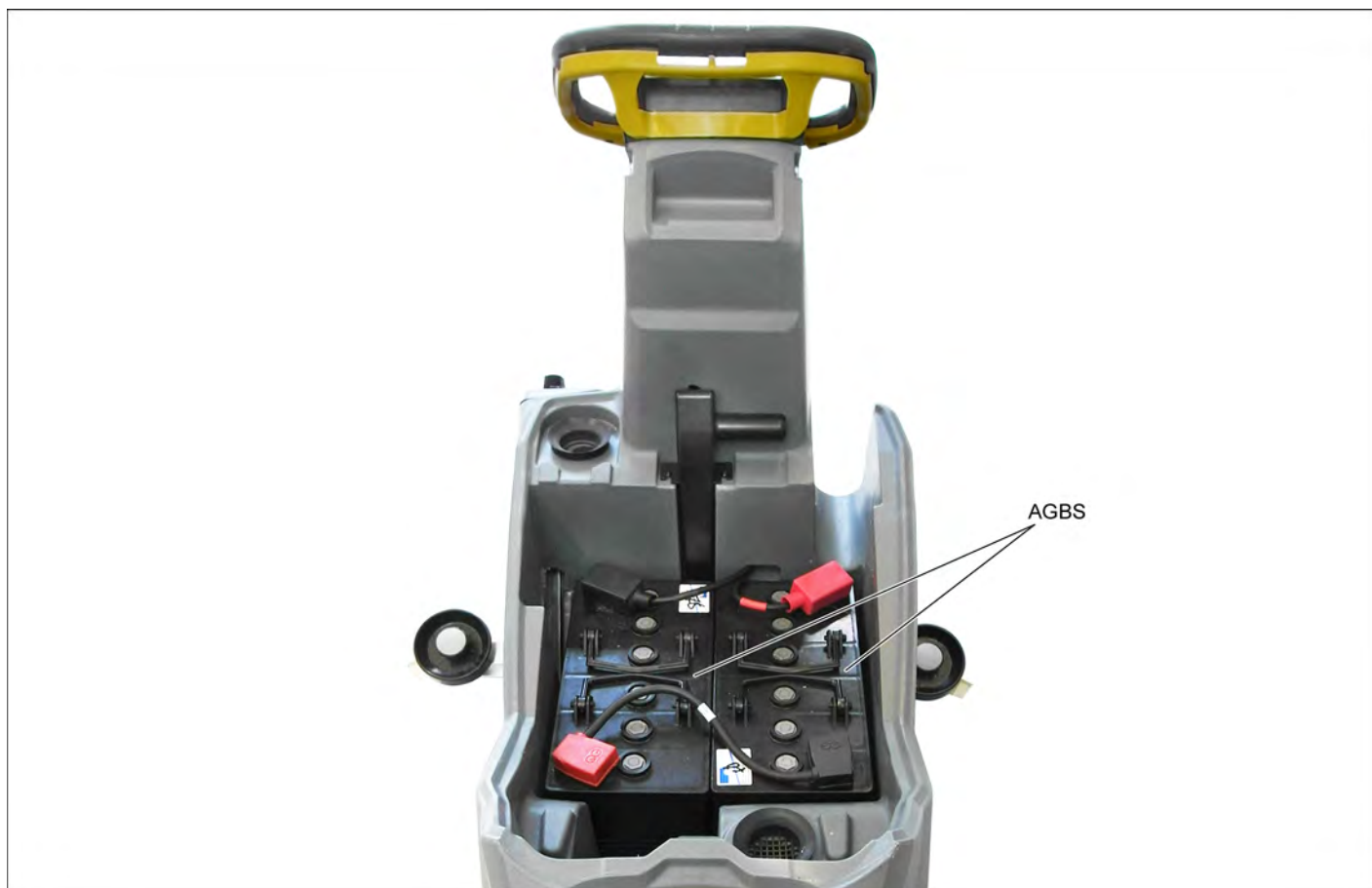
AGBS Uninstall / install batteries
