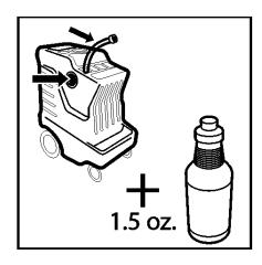
2. To fill Use fill hose or pour directly into solution tank. Use COLD WATER. Add 1 ½ oz of Compass-Rinse TM to each full solution tank.
