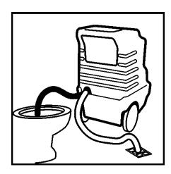
10. Drain machine at proper disposal areas. Use pressure gun to rinse and clean recovery tank.
