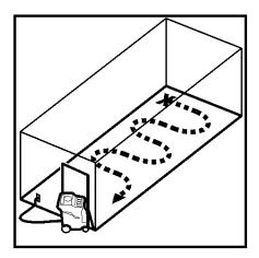
Position the machine in the door way, lock front casters. Start at furthest point in the room and work towards the door.
