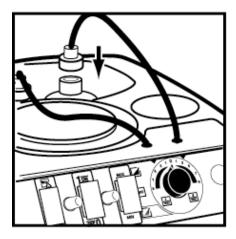
3. Attach the adapter cap and intake hose to the Chemical bottle. Refer to the Chemical Label for the desired dilution.
