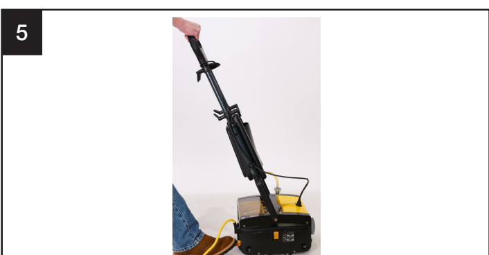
5 Start the machine by pressing the handle release pedal and pulling the handle back.
