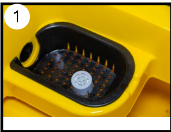
The Bromine tablet holder is located in the debris tray inside the recovery tank
