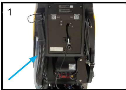
1 Check sight gage hose for solution level
