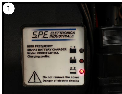
On-board charger LEDs
