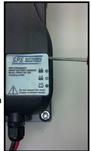
Use small screw driver to lift label off charger
