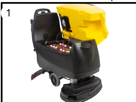
Fully open position allowing access to battery compartment
