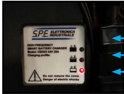
Charging indication LEDs
