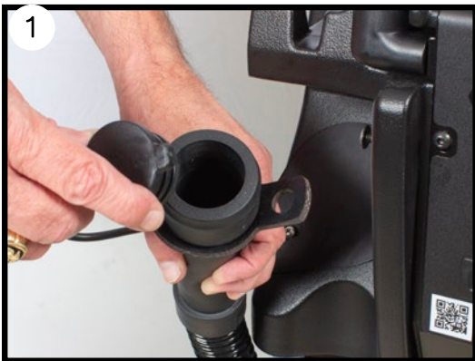
Check for clog in the restriction collar
