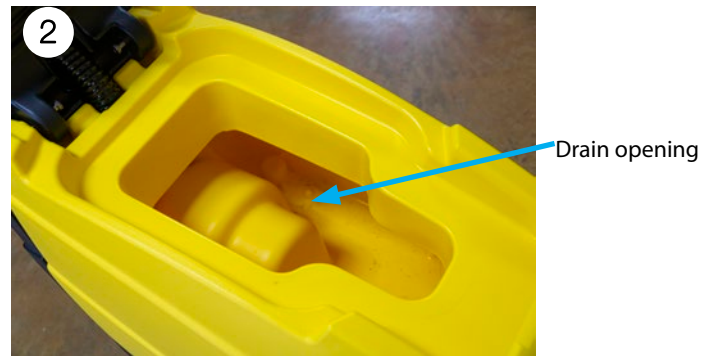
Check for clog in the recovery tank at the drain opening
