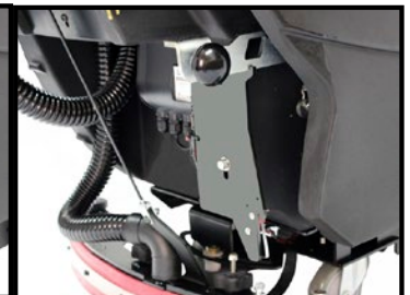
Locking in high down pressure setting by lifting foot lever
