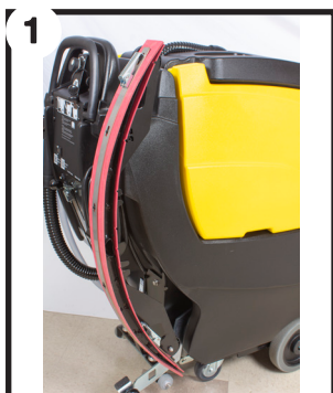
Squeegee assembly in transport position
