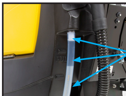
Sight gage hose released from press fitting
