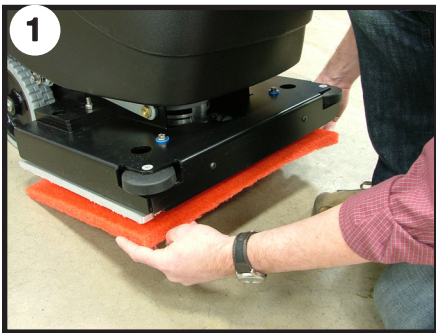
1 Align the front corners of the pad and press to adhere
