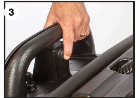
Reverse switch is easily reached with fingertip
