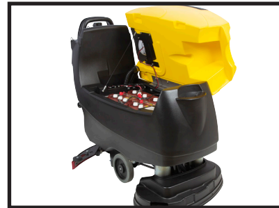
Recovery tank shown in fully open position
