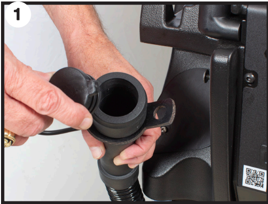
Check for clog in the restriction collar
