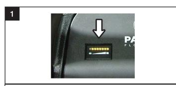
Ensure batteries are fully charged before operating the unit. Refer to the Operations and Maintenance manual for complete charging instructions.
