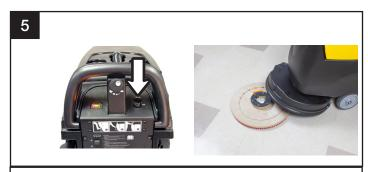
Turn the unit ON using the key switch. Push or drive it into position so that the unit's scrub head is centered over the pad drivers or brushes.
