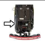
The sight gage hose performs double-duty as the solution drain hose as well. You simply slide the hose off the press fitting and lower the hose to a drain or mop sink.
