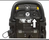
Turn the key to the ON position. You will see the battery meter on the left side of the upper control panel light up to show the battery charge level.
