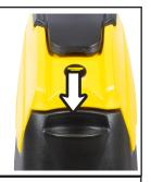
Water and cleaning detergent can be added to the unit's rear hose fill port, located to the left of the control panel. There is also a front fill port that is able to accept hose or bucket filling. Water temperature should not exceed 120°F (50°C).
