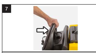
The operation is completed by quickly pulsing the activation trigger. This will "click on" the pad drivers or brushes. If the pad drivers or brushes do not quickly engage, do not continue pressing the activation trigger. Realign the scrub deck and try the procedure again. When you have the scrub deck aligned properly, you should see a noticeable drop of the scrub deck when lowered and the bristle skirt on the shroud should almost be touching the floor.
