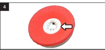
Squeeze center lock wires inward and press center lock down, tab side first, compressing the pad and then release the wires so that they lock in place holding the pad. Repeat for the other pad driver.
