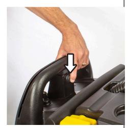
To begin scrubbing, engage the handle trigger. The trigger activates solution flow, the brush motor and traction drive. Speed control is easily thumb adjusted and the reverse can be depressed with your fingers on the back side of the control housing.
