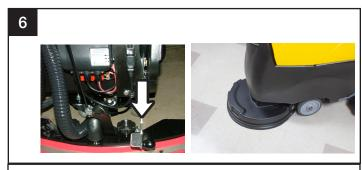
Using the foot pedal, lower the scrub deck down onto the pad drivers or brushes by depressing the pedal while shifting it to the right. Once clear of the lower notch, lifting your foot will lower the scrub deck. Make sure that the shroud completely covers the pad drivers or brushes in the lowered position. Should the shroud be resting on a portion of the pad drivers or brushes, the head is not centered and will not attach properly.
