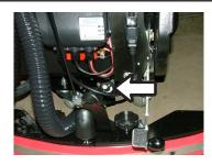
The solution flow rate is adjusted by a control located at the lower rear of the machine.
