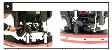
Align the squeegee assembly retention slots with the easy-grip knobs then tighten until secure.
