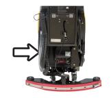
The sight gage hose performs double-duty as the solution drain hose as well. You simply slide the hose off the press fitting and lower the hose to a drain or mop sink.
