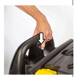
To begin scrubbing, engage the handle trigger. The trigger activates solution flow, the brush motor and traction drive, if equipped. Speed control is easily thumb adjusted and the reverse can be depressed with your fingers on the back side of the control housing.
