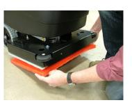
To attach the pad, align the front corners of the pad to the front corners of the orbital drive plate and press to attach. Use the foot pedal to lower the scrub deck down onto the pad ensuring alignment from front-to-back and side-to-side.
