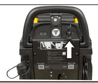
Turn the key to the ON position. You will see the battery meter on the left side of the upper control panel light up to show the battery charge level. 5
