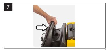
The operation is completed by quickly pulsing the activation trigger. This will "click on" the pad driver or brush. If the pad driver or brush do not quickly engage, do not continue pressing the activation trigger. Realign the scrub deck and try the procedure again. When you have the scrub deck aligned properly, you should see a noticeable drop of the scrub deck when lowered and the bristle skirt on the shroud should almost be touching the floor.
