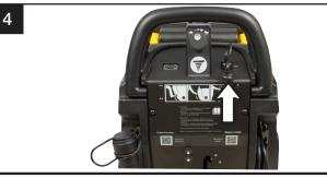
Turn the key to the ON position. You will see the battery meter on the left side of the upper control panel light up to show the battery charge level.
