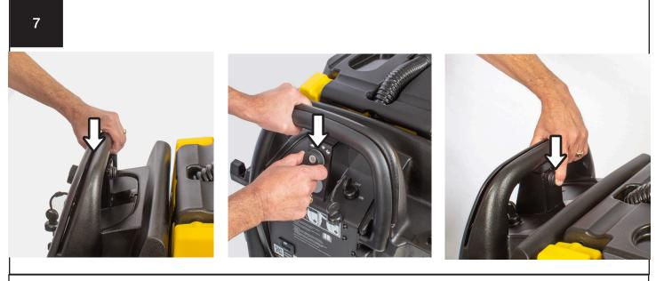
To begin scrubbing, engage the handle trigger. The trigger activates solution flow, the brush motor and traction drive, if equipped. Speed control is easily thumb adjusted and the reverse can be depressed with your fingers on the back side of the control housing.
