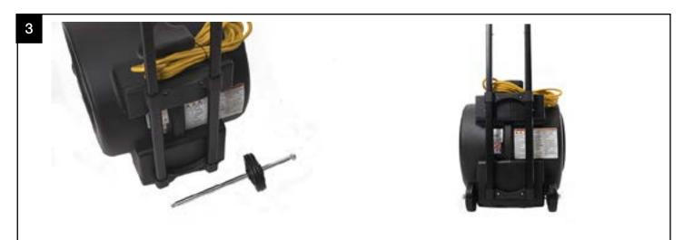
Hand tighten one nut at end of axle then slide one wheel onto axle. Push axle through hole in blower housing then attach other wheel and nut. Using two wrenches, tighten the two nuts until fully threaded.
