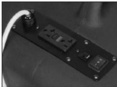
2 position switch and daisy-chained outlets
