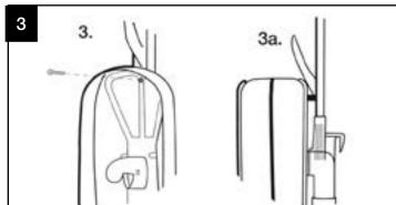
Slide screw through plastic Cord Hook from the inside of Cloth Bag. Align screw with hole in Handle Tube. Tighten screw.
