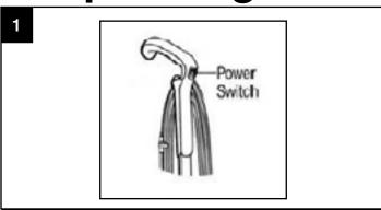
The Power Switch is located in the Handle of the unit. Push down (I) to turn ON. Push up (O) to turn OFF.
