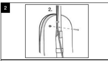
Hold the hex nut in front of the Connector in the hex shaped cavity while inserting the screw with your finger from the back. Tighten the screw while placing your finger over the hex cavity to hold the hex nut in place. After a few turns, tighten further with a Phillips head screwdriver. Do not overtighten.
