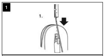
Slide the handle Tube into the Connector, aligning the hole in the Handle Tube with the molded hole at the top of the Connector.
