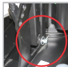
Remove the Handle Mounting Pin w/o Tools
