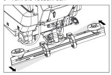
→ Tighten the wing screws.
