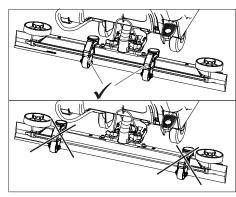
Check if the height adjustment is mounted on the inside of the vacuum bar. When the height adjustment is mounted on the outside, the vacuum bar gets caught at the bottom of the appliance.
