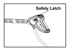
**STEP 5:** Lock trigger gun safety lever to prevent unintentional pulling of trigger.
