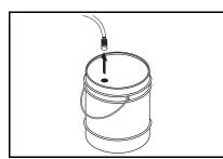
**STEP 1:** Remove detergent suction tube from container and insert into 1 gallon of fresh water. Turn variable pressure wand handle for low pressure or connect the black detergent nozzle. Pull trigger on spray gun and siphon water for one minute.
