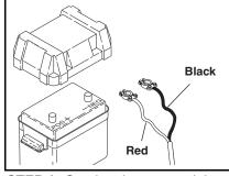
**STEP 6:** On electric start models, you will need to install a battery making sure that the red cable is attached to the positive terminal. Use a Group U1 garden tractor style type of battery rated for 300 CCA (battery not included).
