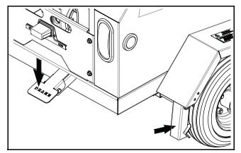
To set the brake, press down on the brake pedal until it engages on the back tires.
