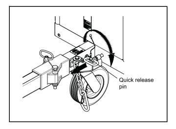
**STEP 1:** Release the quick release pin by rotating it clock wise. Pull Quick release pin from receptacle. Rotate the caster clockwise.
