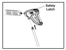
**STEP 3:** Attach wand to spray gun using teflon tape on threads to prevent leakage. Attach swivel connector on discharge hose to spray gun using teflon tape on threads. Attach swivel connector on high pressure hose to spray gun using teflon tape on threads. Engage safety latch to prevent from triggering gun.
