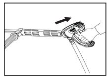
**STEP 4:** Turn garden hose water off. Open the spray gun to relieve remaining pressure.
