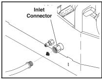
**STEP 1:** Attach a 5/8" garden hose to inlet connector. Minimum flow should be 5 gpm.
