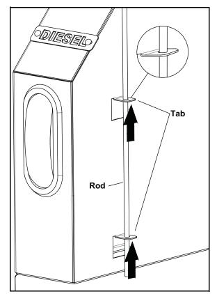
Slide the rod through both holes in the tabs. To secure rod, bend both tabs up slightly, until the rod does not move freely. (See Hose Box and Fuel Tank pages for fastener part numbers.)
