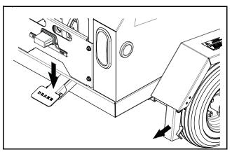
To release the brake, push the center of the brake to release see that it has disengaged from the back tire.
