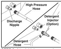
**STEP 2:** Attach high pressure hose to discharge nipple using quick coupler. Lock coupler securely into place by pulling back coupler collar and inserting it onto discharge nipple, then pushing collar forward to lock in place.
