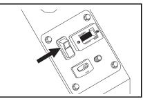
**STEP 2:** Turn burner switch off and continue spraying water, allowing the water to cool. After water has cooled to less than 100°F, turn off engine. Protect from freezing.
