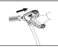
**STEP 2:** Grip spray gun handle securely and pull trigger.
