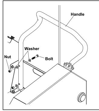
Align the 4 holes in the handle with the holes in the back plate, install the fasteners and washers supplied. (See Hose Box and Fuel Tank pages for fastener part numbers.)
