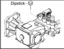
**STEP 4:** Check oil level on sight glass on backside of pump. Oil should be visible one-half way up sight glass (10-40W non-foaming). The oil level can also be checked by using the dipstick on the top of the pump.
