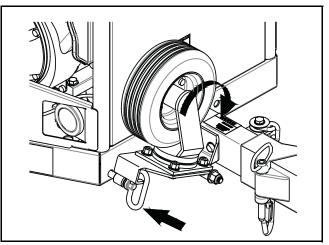
**STEP 2**: Insert quick release pin in receptacle. Lock quick release pin in place by rotating pin counter clockwise. Reverse step to lower caster.
