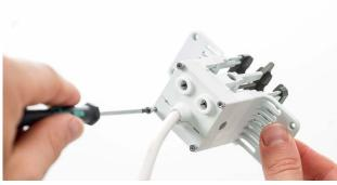
**Caution:** Overtightening the M2.5x75 bolts can damage the print head. This puts more pressure on the linear bearings, causing excessive wear of these parts. Only use the 0.15 Nm torque screwdriver.
