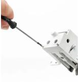
**Caution:** Overtightening the M2.5x75 bolts can damage the print head. This puts more pressure on the linear bearings, causing excessive wear of these parts. Only use the 0.15 Nm torque screwdriver.
