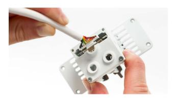
**Tip:** If the cable does not click into place, use the hex screwdriver to push it completely into the connector.
