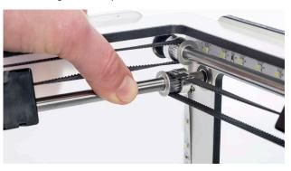
**Caution:** The orientation of this pulley is different from the others. All other pulleys have their wide side facing **towards** the frame, this pulley has its wide side facing away from the frame.
