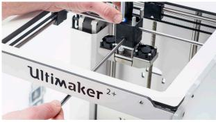
**Tip:** The X axles are only secured on one side. Be careful not to push the axles out of the frame when moving the front and back sliding blocks. Hold the axle in place while adjusting the sliding block's position.
