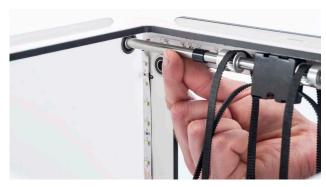
**Tip:** Make sure the axle is in the middle of both bearings and push the pulleys against the frame. This helps to keep the axle in place before the pulleys are tightened.
