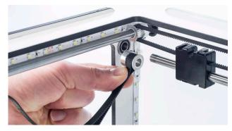
**Tip:** Make sure the axle is fully inserted into the front panel and push the pulleys against the frame. This helps to keep the axle in place before the pulleys are tightened.
