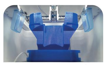
Large flexible parts in TPU 95A to TPU 70A
