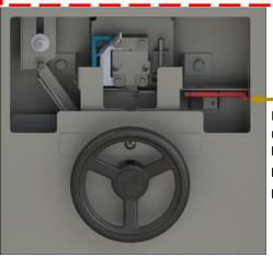
Red Lever position during internal release/mechanism override DO NOT MOVE RED LEVER TO POSITION SHOWN DURING PANIC ROOM LOCK-IN
