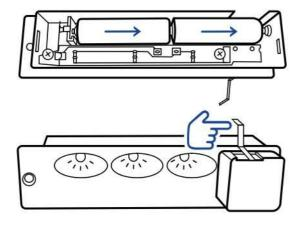
5.3. **Install the LED light** by sliding in the right (lever) side first, then tide in the crew.
