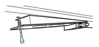
5.2. Install 2 new AA batteries and **test by pressing the lever down.** The light should turn on.
