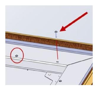
Lift rear frame from vault door and set aside, remove shipping spacers. (Refer to Figure 3):
