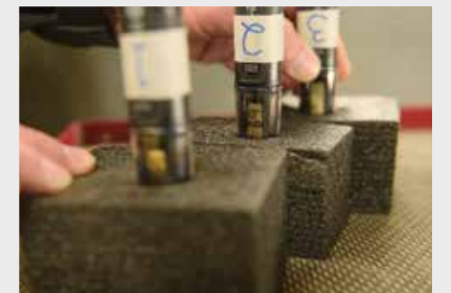
Temperature gauges being prepped for test
