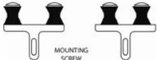
USE ONE OR TWO O-RINGS ON EACH SPACER TUBE
