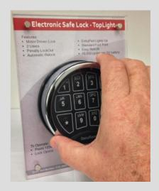
Step 6: Place the ring back over the EntryPad by engaging the keys on the ring with the slots on the EntryPad base. Turn clockwise to lock in place.
