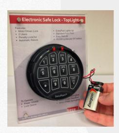
Step 4: Remove the battery from the compartment and unclip the battery terminals.
