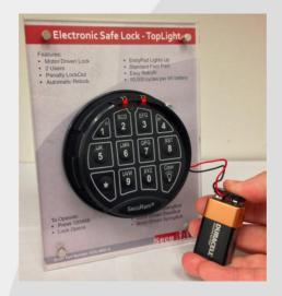
Step 5: Snap on a new battery. We recommend either Duracell or Energizer standard alkaline batteries
