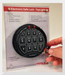
Step 3: Push the battery from the left side of the compartment and slide out.
