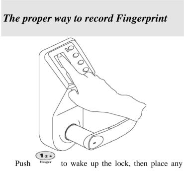
finger you wish to use on the window panel for fingerprint enrollment. Finger must be placed parallel with the digital pad. It is advisable to press with a little pressure against the glass panel window during enrolling as this will provide a larger scanned finger surface area to ensure proper data entry and smooth operation of the lock.
